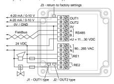
4. To use relay outputs, connect the chosen actuators to the relay terminals RE1 and/or RE2
