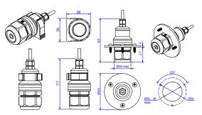
The recommended orientation of sensor probe is vertical with the sensor tip pointing downwards. This prevents possible accumulation of condensed water on the sensor protection filter. The horizontal orientation is also suitable. Avoid upward position of the sensor tip.
